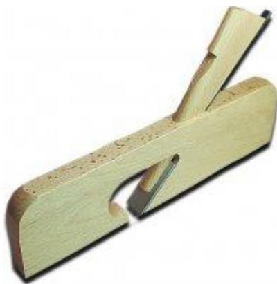
The Rabbet Plane is a narrow plane, which is perfect for planing slots, half slots, sills, or rabbets on doors and window frames. The body is made of high quality beech, both dried down to 10 % moisture. The blade is inserted near the centre of the body, bed angle is 45 degrees and it planes across the entire width of the plane.
